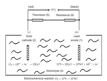
Fig. 3-7: Electrochemical reaction of Oxygen Sensor
